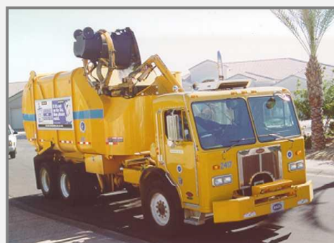
The Automated Sideloader of today. Scottsdale 2000's
