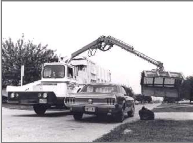
In Texas they tried to automate residential collection by collecting plastic bags from the curb with this boom and claw.
