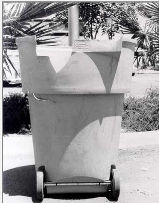
This sight is rare today as the original container designed by Marc Stragier has been refined over the years and rarely fail.
