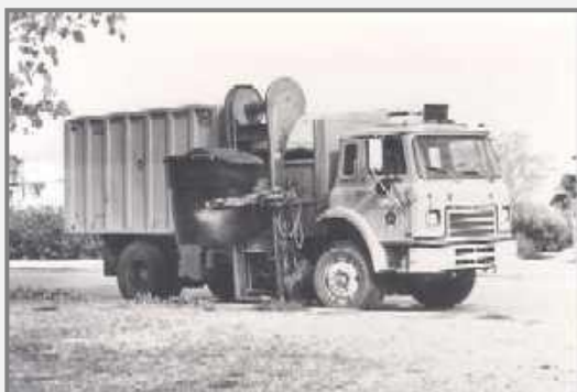
The Automated Sideloader with a "rail" lift arm Scottsdale 1978
